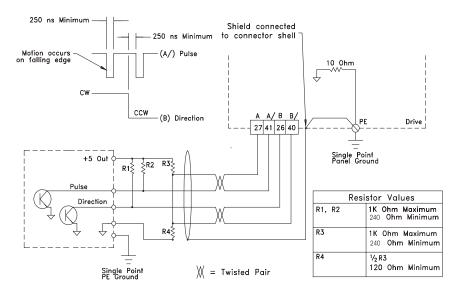
Figure 26: Pulse Mode, Single Ended Output to Differential Input
